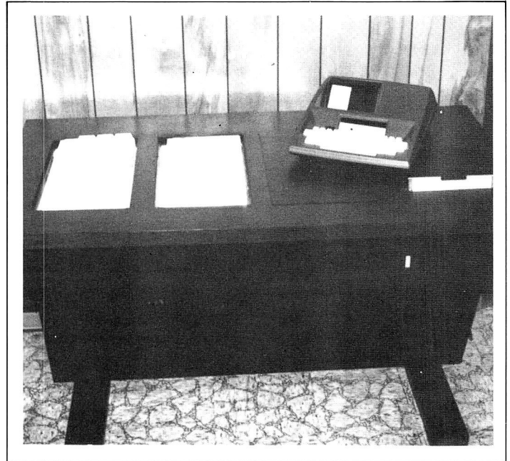
Randomatic desk console, with two recessed selector trays to the left and the AIM 65 controller to the right. The slot in front of the AIM 65 is the punch unit. The power supply and interface are inside the console.
